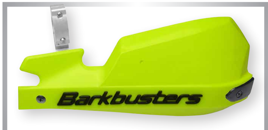
The VPS from Barkbusters is an open-ended handguard with a single-point mount, allowing for quick and easy mounting. It's designed to protect the rider's hands against dirt, rocks and other roost out on the track or trail.
