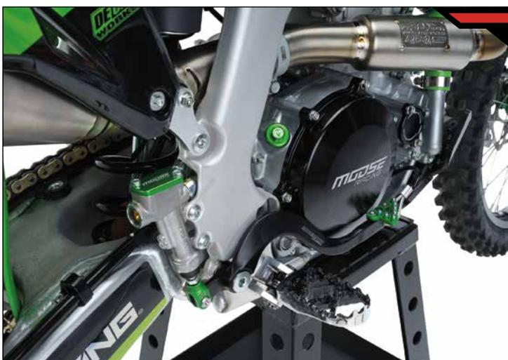
Moose Racing also supplied the upgraded foot controls, including shift lever, brake pedal, hybrid footpegs. Details count on this bike, and this one has them down pat.
