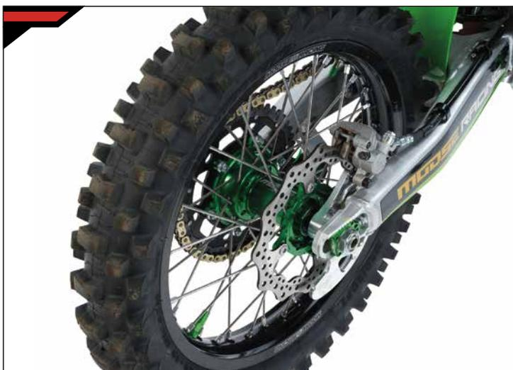
Out back, the Kawi got a Moose Racing dual sprocket, Shark Fin disc guard and RFX rotor.
