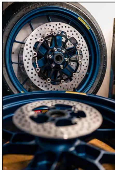
The Halo brake disc pairs the premium-quality stainless steel outer ring with a CNC-machined billet aluminum carrier, which is black anodized for a durable, attractive finish.
