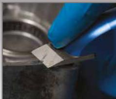
Steel blade included for difficult to remove paper gaskets
