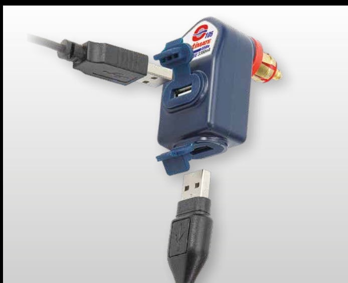
The O-105 is a USB charger that connects to a Ø12mm DIN socket and delivers 3300mA of charge through dual USB-A ports. It's popular with BMW and Triumph motorcycle riders.
