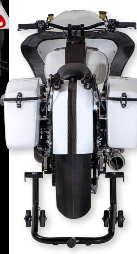
Beginning with an S&S Cycle 124-inch package and a complete Feuling valvetrain upgrade, the engine Alex Fox and the SLYFOX team spec'd out is race-ready. A Bridgestone Racing slick on a 6-inch wide SLYFOX Track-Pro wheel takes the power. It's covered with a SLYFOX carbon fiber fender and flanked with SLYFOX carbon fiber saddlebags and lids.
