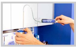
Motion Pro's Pro Fork-Oil Level Tool allows service techs and 'do it yourself' enthusiasts alike to get that critical oil level exactly right every time with no fuss and no mess.
