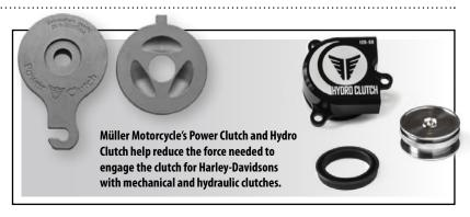
The Hydro Clutch (p/n 1130-0416) provides the same finger-saving service for Twin Cam and M8 models with hydraulic clutches. Müller Motorcycle reports that Twin Cam models get a 35 percent reduction in the force required to engage the clutch lever, while the M8 models have a 45 percent reduction.
