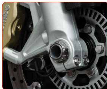
AXLE NUTS | DISC ROTOR BOLTS | AXLE PINCH BOLTS
