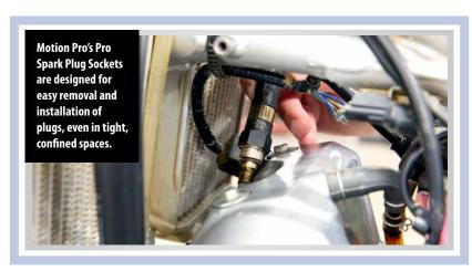
Pro Spark Plug Sockets are versatile in complementary tools, designed to take a 17mm combo wrench for extratight clearance situations, or a 3/8-inch square drive with a ratchet for more standard jobs. Much like all Motion Pro tools, Pro Spark Plug sockets are constructed to last, utilizing strong tool steel material, making it easy for Motion Pro to cover these under a lifetime limited warranty.
