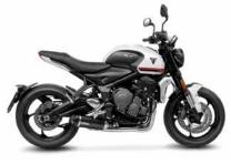
1. The exhaust device fulfills the ECE-R92 and EU 134/2014 directives only if the catalyzed link pipe is installed. For the validity of the homologation according to  $the \ ECE-R92 \ and \ EU\ 134/2014 \ directives \ concerning \ noise \ and \ polluting \ emissions, the installation of the optional \ catalyzed \ fitting \ is \ required.$
