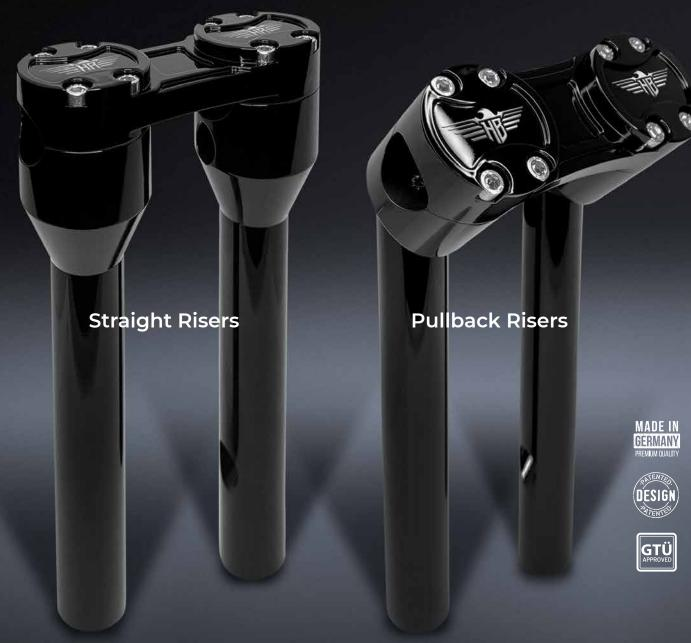
Top clamp out of one piece for maximum stability in 4 colours. Risers in high gloss black or silver anodized, in 6, 8, 10 and 12 inch.
