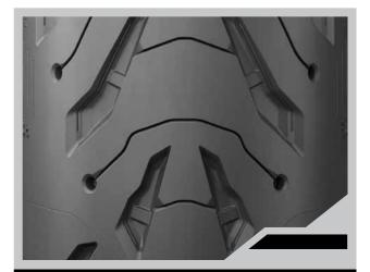
The sipes on the MICHELIN Road 6 are designed to widen over the service life of the tire to maintain the tire's water dissipation capacity.
