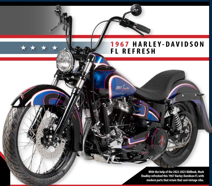
That everyday usable, friendly bike theme carried through to the FL's chassis upgrade. Up front the five-decade-old suspension was replaced with an all-new system Mark pieced together using triple-trees from a Harley Deuce, Drag Specialties upper tubes and Dyna Wide Glide lowers. A vast improvement in ride and handling, the setup also netted a disc front brake.
