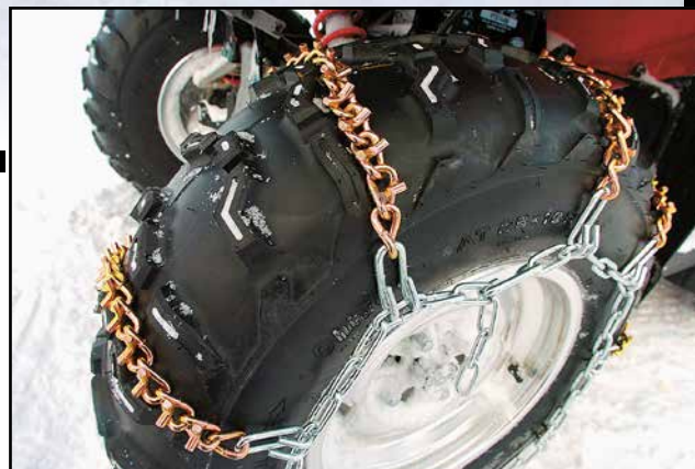
Moose Utility Division has four sizes of tire chains available, which means nearly any ATV or UTV can be outfitted with a set. These chains help tires maintain grip in slippery snow and ice.
