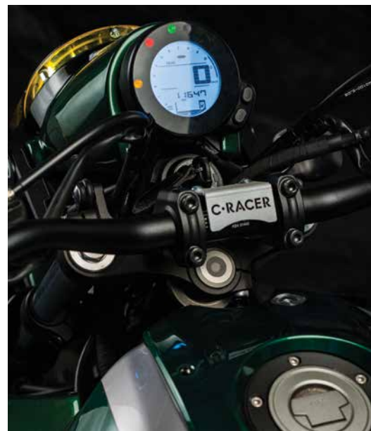
Speedometer Holder with Headlight Cover 2210-0537 ABS Plastic & Black powder coated metal
